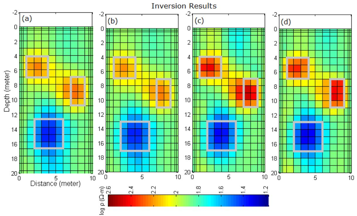
**Figure 2.** Inversion results of (a) AMN array, (b) ABM array, (c) A-BMN array and (d) joint inversion of all arrays data sets
