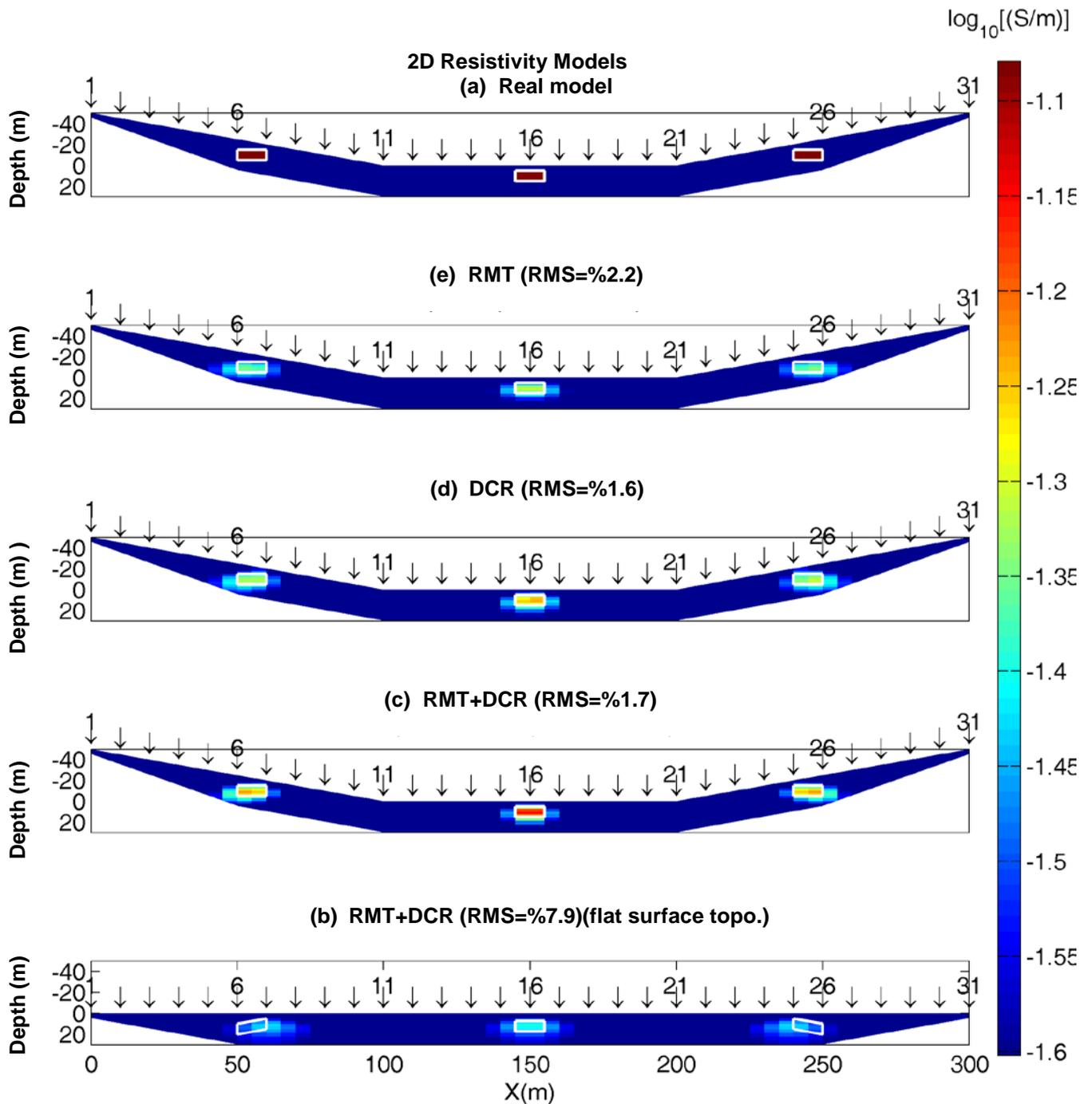
**Figure 1.** (a) 2D resistivity model (slope is 26°). Inversion results of different data: (b) RMT data inversion result, (c) DCR data inversion result, (d) Joint inversion result of RMT and DCR data, (e) Joint inversion result of RMT and DCR data assuming flat surface topography.
