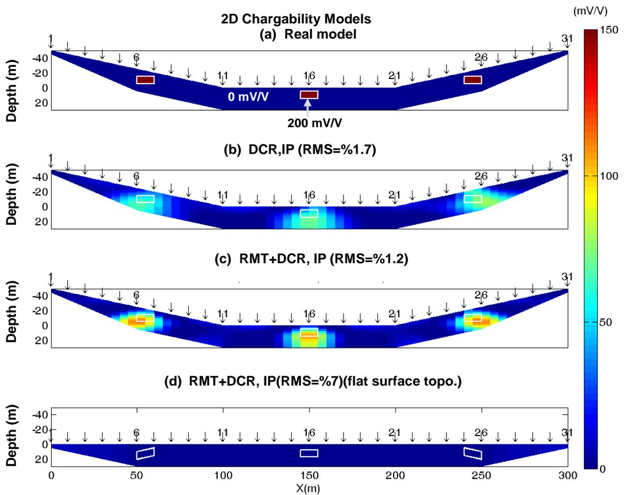
**Figure 2.** (a) 2D chargeability model (slope is  $26^\circ$ ). Inversion results of apparent chargeability data: (b) inversion with the resistivity model in Fig.1c (c) inversion with the resistivity model in Fig.1d, (e) (b) inversion with the resistivity model in Fig.1e
